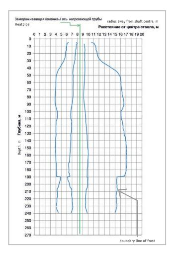
the strata was initially affected mainly by the natural ground heat and so tended to recede more slowly. The freeze boundary facing the shaft column was subjected to the heat effect of the shaft ventilation system.
