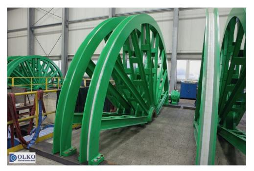
Well prepared to load: rope sheaves
