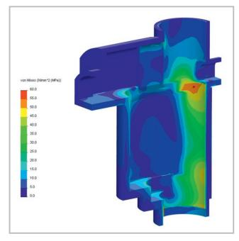
Von Mises- stress (O until 60 MPa) at the designed shaft landing site
