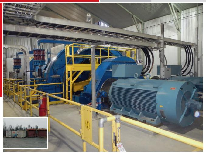
Pic. left: Winch of Nordberg prior purchasing Large pic.: Nordberg-winch after assembly and commissioning with walkway surfaces, stages and new alternating current motors
