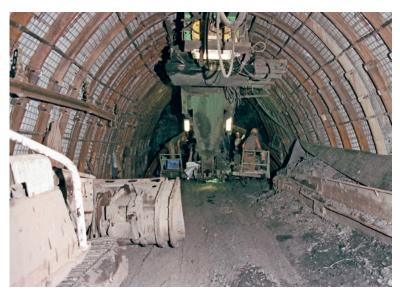
GTA stage AMG 2800, loader K 313 S and crusher with chain conveyor in a drift
