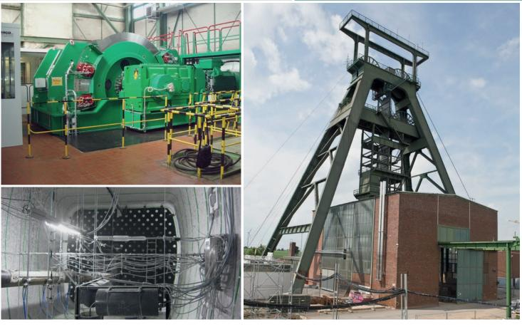
Pic. top left: Hoist engine, a product of the OLKO-Maschinentechnik Pic. bottom left: Construction of sealing dam in rock salt strata Pic. right: Shaft refurbishment during the construction of the permanent disposal site Konrad
