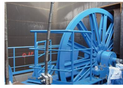
Hoisting sheave platform with rope sheave
