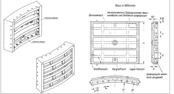
Pic. left: Scheme of the Russian cast iron tubbing segment, i.e. 7.0-120 GG35
