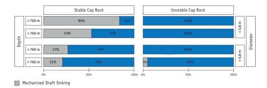
Figure 7: Sinking method in relation to strata stability, shaft depth and diameter.
