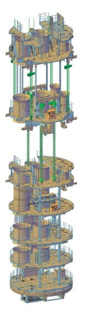
Scheme of the seven-deck shaft platform: working and support unit The sinking cycle includes the following main operations:
