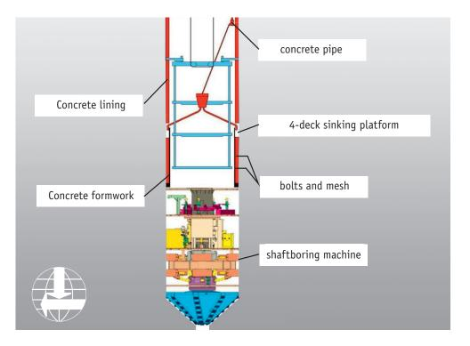
machine is used to apply an immediate supporting layer to the newly exposed side walls. The machine is about 15 m in height and has an overall weight of 350 t.
