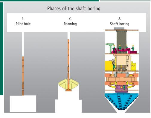
The three phases of shaft drilling with pilot hole manufacturing
