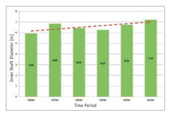
Figure 4: Developments in average shaft diameter.
