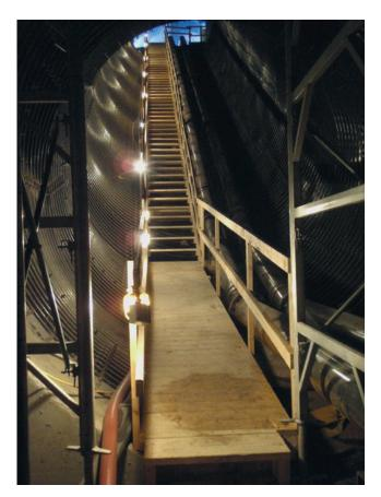
Brine pipes in the air drift beneath shaft head
