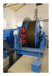
Hoisting engine in the winch house with support frame and gear support
