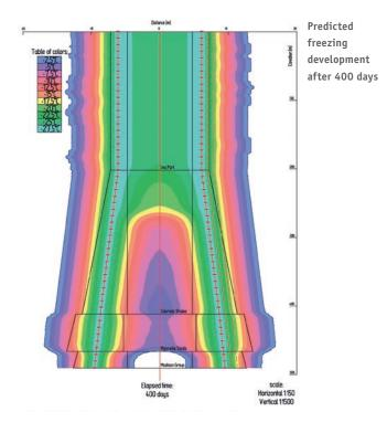
In the initial stages of freezing, the 5  $\times$  800 kW plants froze one shaft while the 3  $\times$  1250 kW plants froze the other. Once the freeze load subsided, the system was reconfigured and both shafts were cooled by the 3  $\times$  1250 kW plants.
