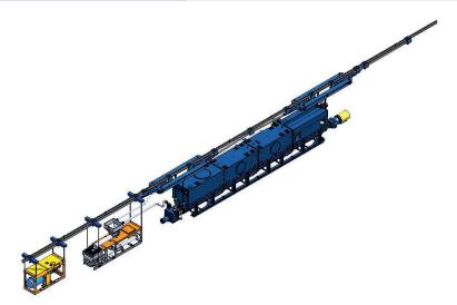
Overview of an on-site plant on an overhead monorail rail track
