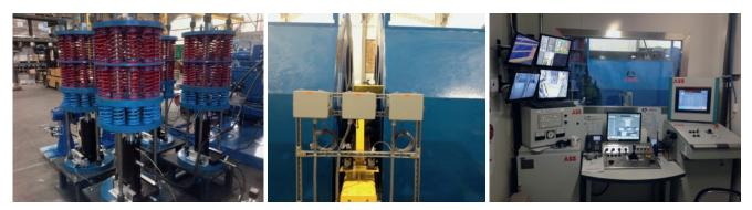
New Siemag drives for drum brake during test phase with new hydraulic aggregate
