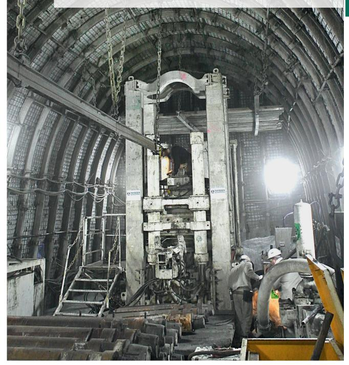
Raise drilling machine HG 250 in the drilling chamber I 547
