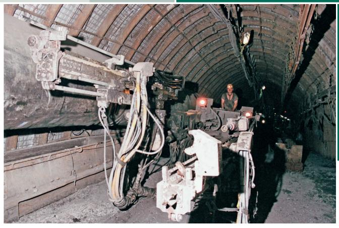
Drilling jumbo BTRK-2 for drilling blasting and block (Hilti) holes
