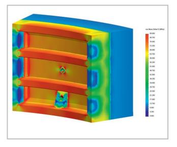
Results of the stress analysis, Tubbing 7.0-120, thickness of concrete 58 cm, depth 642,35 m
