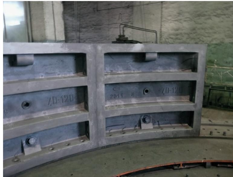
Test assembly of the cast iron tubing segment at the surface.
