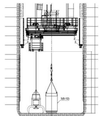
Schematic view at the rock support and shaft lining operation
