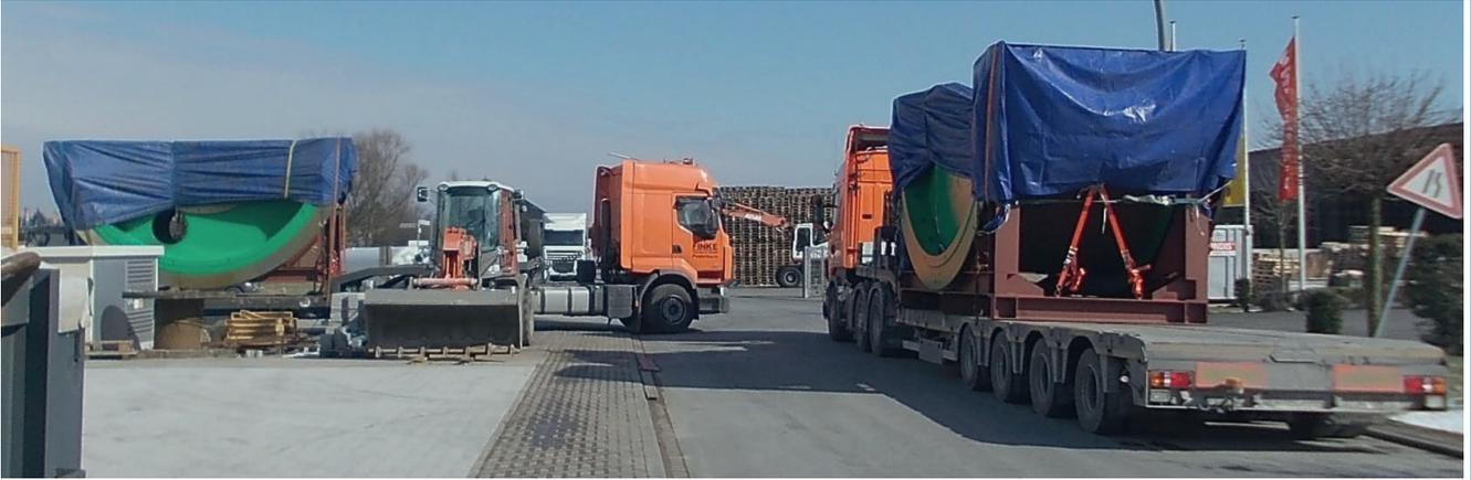
Visible comparative sizes - a half rope drum can fit on a truck
