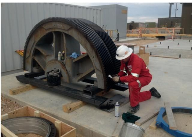
Preparing for mounting a rope sheave half
