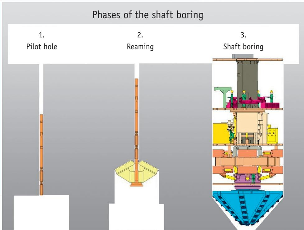
The three phases of shaft drilling with pilot hole manufacturing
