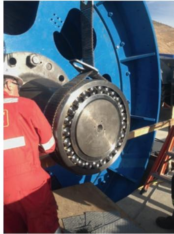
Mounting of the bearing on the main shaft
