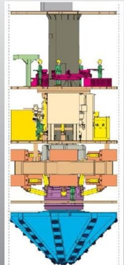
Shaft drilling machine on pilot hole: performance data and schematic design configuration
