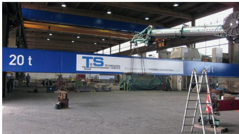
Assembly of the 20 tons crane after complete redevelopment
