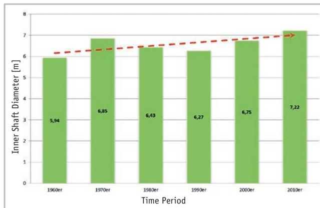
Figure 4: Developments in average shaft diameter.
