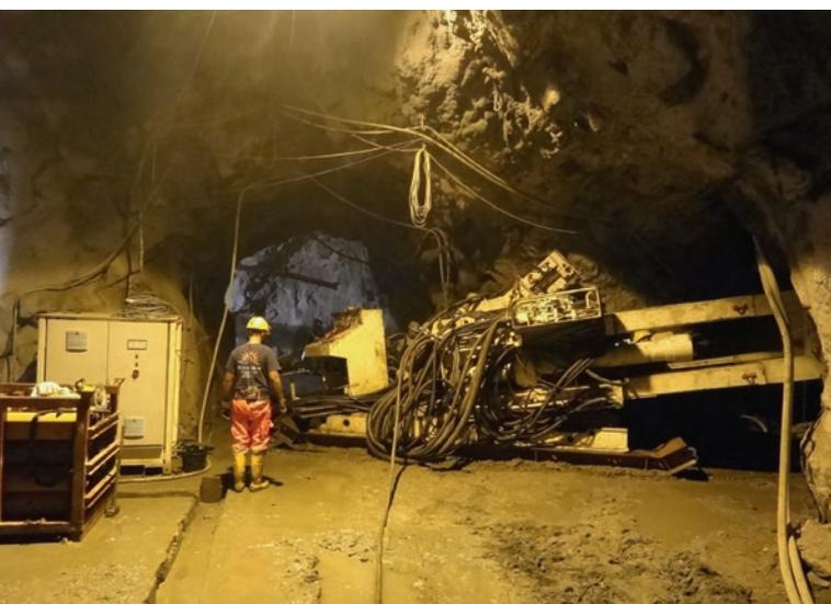
ground. In pursuit of this target THYSSEN SCHACHTBAU was commissioned to introduce the latest fully-mechanised raise-boring technology in place of the accident-prone and dangerous Alimak based shaft sinking equipment.
