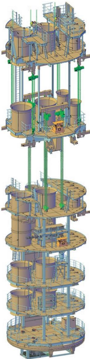
Scheme of the seven-deck shaft platform: working and support unit
