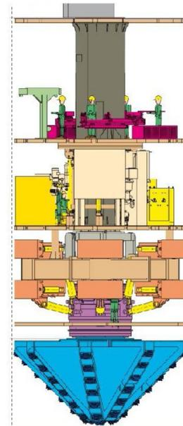
Figure 6: New Herrenknecht shaft boring machine for pilot hole-based projects
