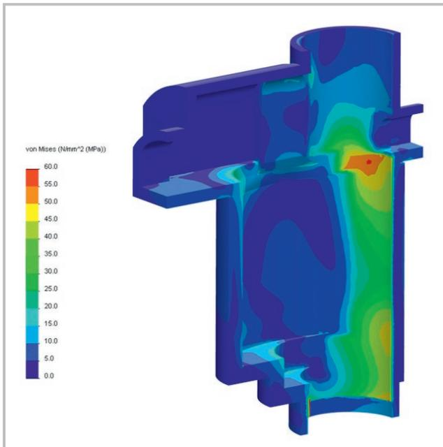
Von Mises- stress (0 until 60 MPa) at the designed shaft landing site
