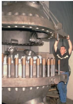
Pic. left: Assembly of the high-pressure outer jacket after revision works of the 180 MW turbine, Hermann Wenzel power plant of ThyssenKrupp AG, TKSE
