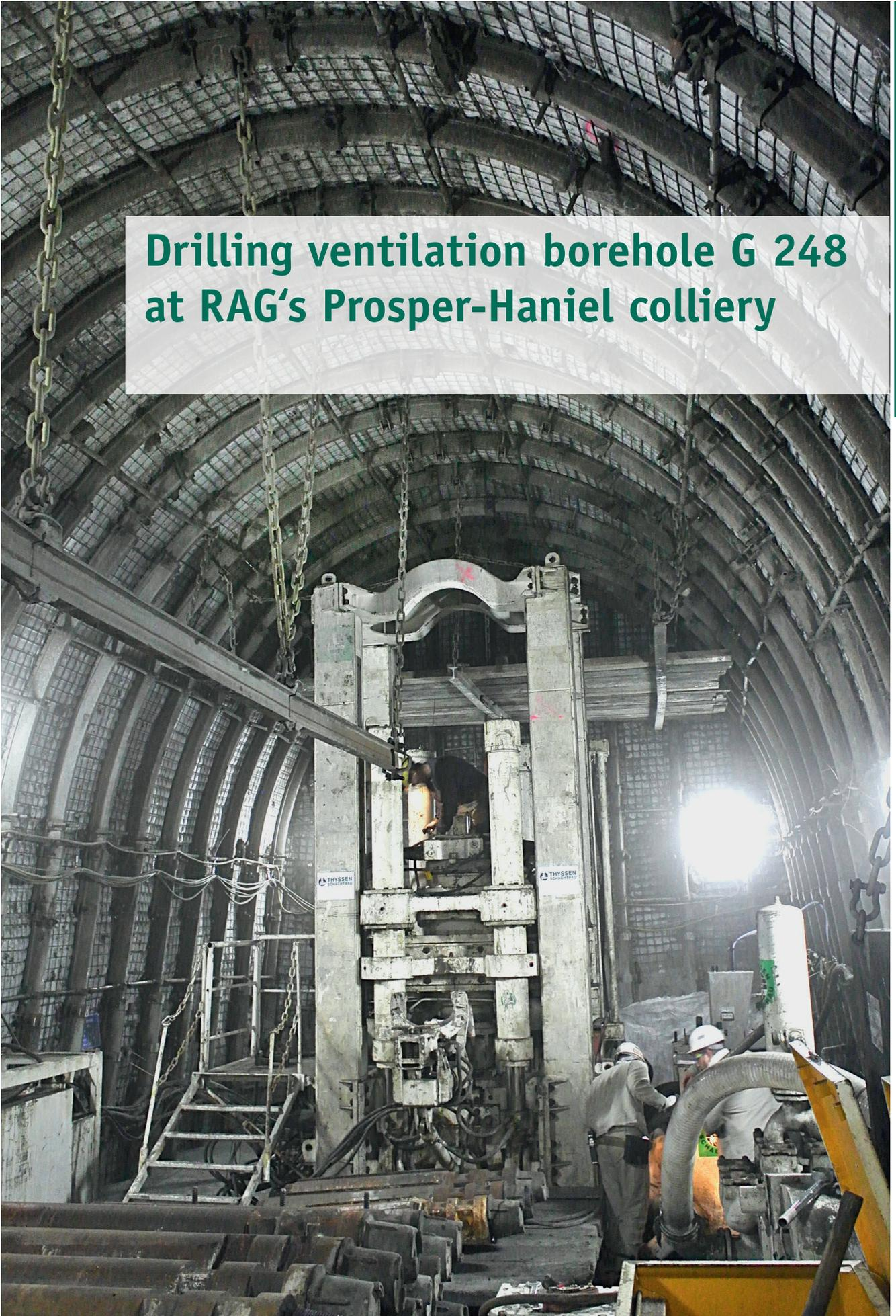
Raise drilling machine HG 250 in the drilling chamber I 547
