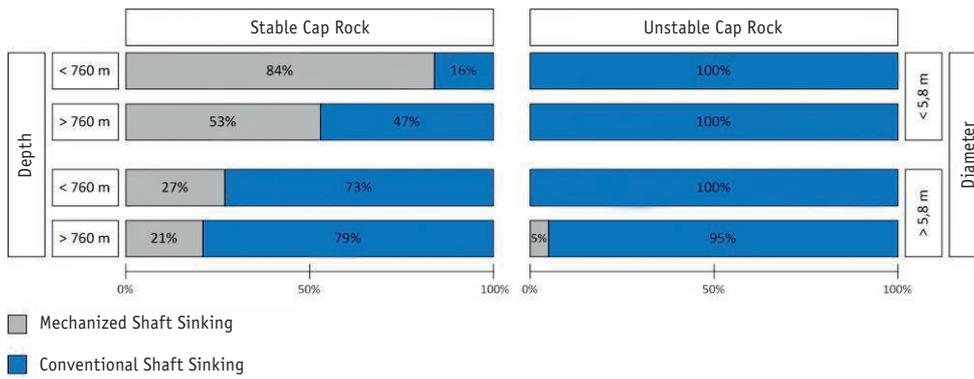
Figure 7: Sinking method in relation to strata stability, shaft depth and diameter.
