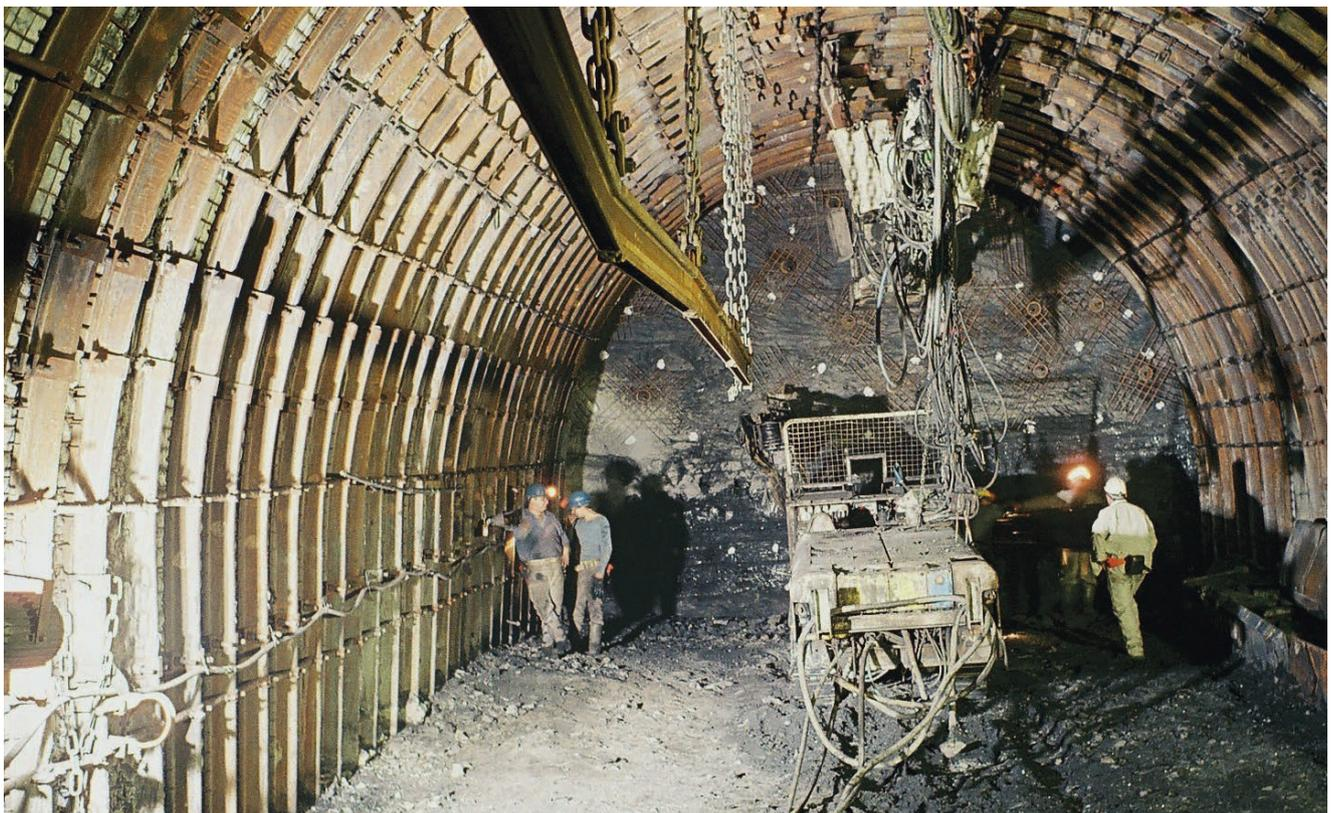
The high risk of gas outbursts has compelled the mine to employ systematic exploratory drilling in the drivage zones, the results of which then determine the weekly rates of advance. Because of the gas hazard roadheading machines are not used in the conventional development zones.
