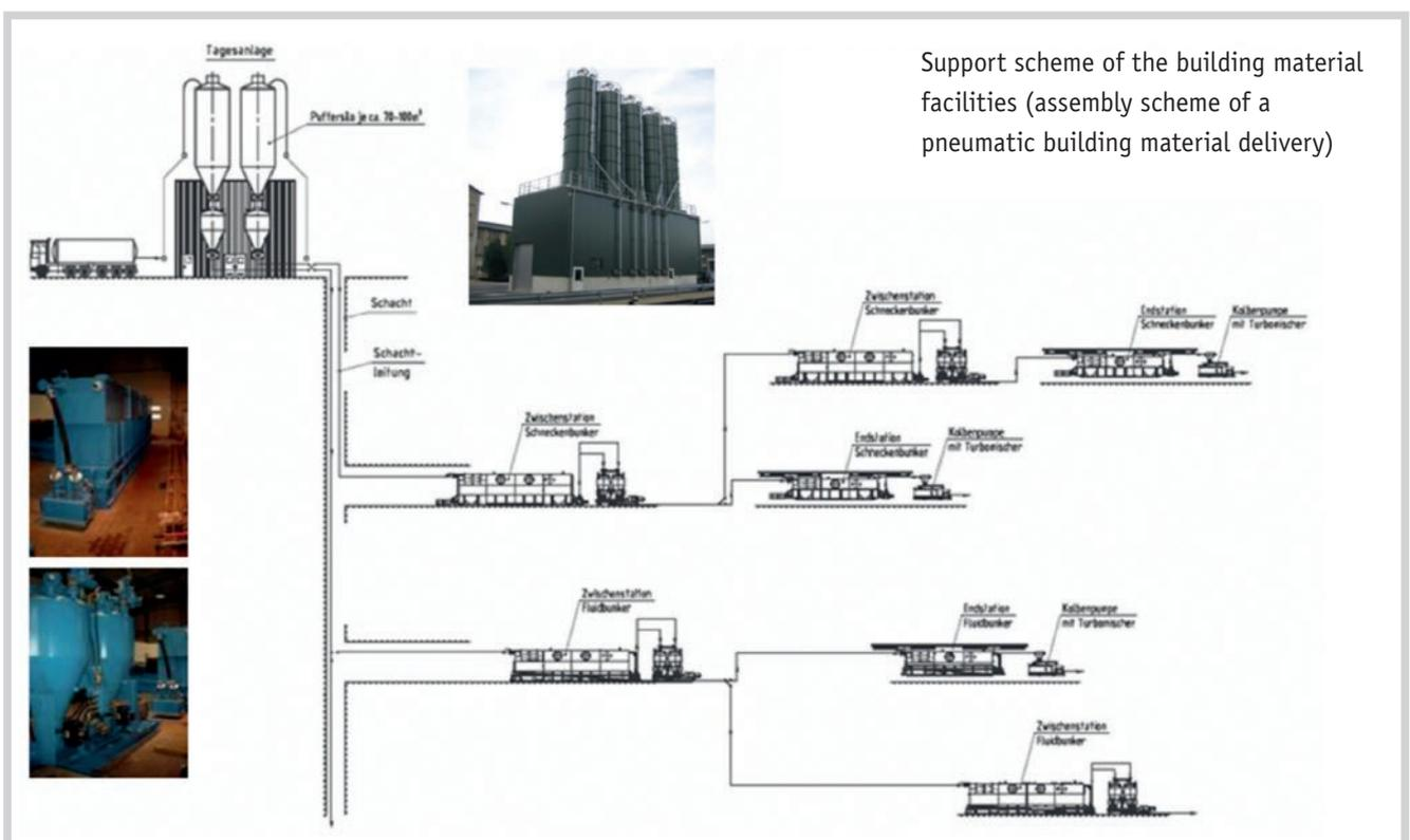
Support scheme of the building material facilities (assembly scheme of a pneumatic building material delivery)
