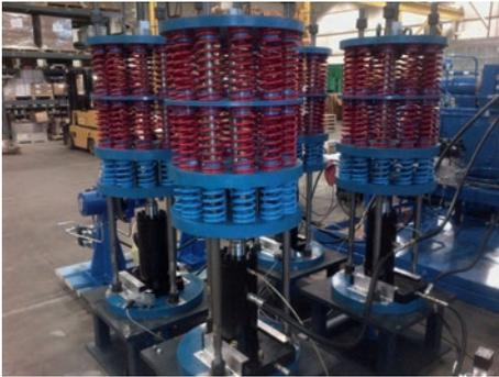
New Siemag drives for drum brake during test phase with new hydraulic aggregate
