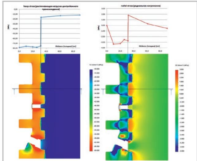
Value and behavior of the hoop and radial stress within the cast iron tubbing element and the back fill concrete
