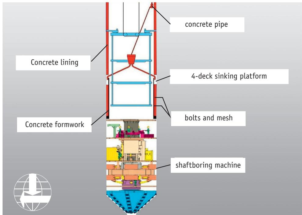
machine is used to apply an immediate supporting layer to the newly exposed side walls. The machine is about 15 m in height and has an overall weight of 350 t.
