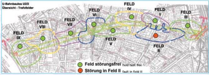
Figure 3: Layout of pumping sectors
