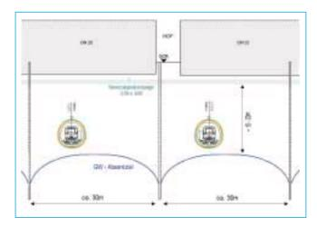
Figure 4: Groundwater Lowering operation
