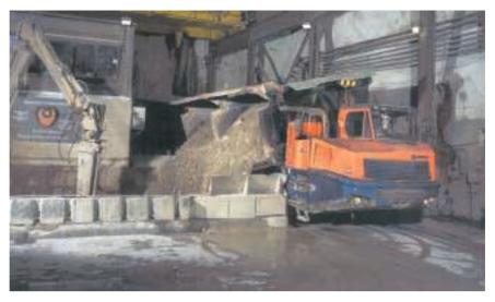
An 80 ton side-dumping Tamrock Supra truck tipping its load into the underground crusher in a matter of seconds
