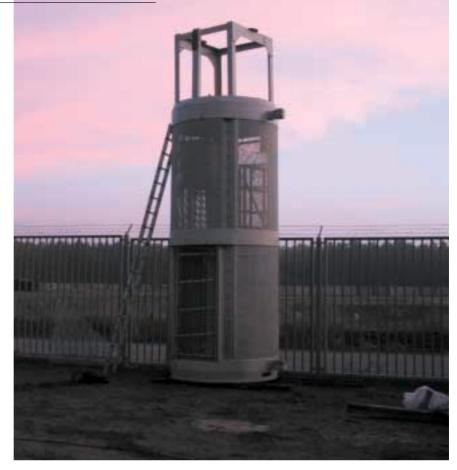
Mini manwinding cage after refurbishment
