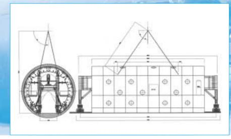
Cross- and longitudinal section of the tunnel formwork car
